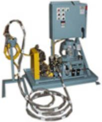
The Model 201-05 is driven by a dependable hydraulic motor to bring process control to high volume applications. Completely portable and using the M-6500 series pumps, the Model 201 is capable of generating flow rates up to 5 lbs/min. The Model 201-05 is suitable for either manual or robotic operations dispensing high viscosity windshield adhesives.
