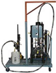
Economical, compact and portable, the Model 500-10 (Formerly M500MMS) is electric driven. This unit is designed specifically to pump methacrylate adhesives at ratios from 1:1 to 10:1 and can achieve flow rates as high as 3 lbs/min with up to 3000 psi material pressure. The electric drive makes it ideal for precision dispensing in manual, automatic or robotic applications.
