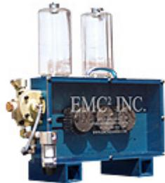
This version of rotary metering is small enough to mount on a robot arm, bringing precision metering to a new level. Featuring our M-3900 series pumps and a servo motor drive, this unit is ideal for small precision beads. Since the Model 500-20 is mounted close to the work piece, it is possible to make rapid flow rate changes during the application. It is designed for smaller volumes, but can achieve flow rates as high as 1 lb/min with up to 3000 psi material pressure.
