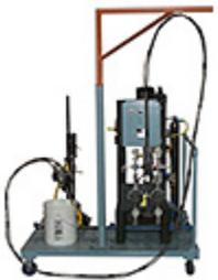
Economical, compact and portable, the Model 100-10 (Formerly M100MMS) is completely air driven. This unit is designed specifically to pump methacrylate adhesives at ratios from 1:1 to 10:1 and can achieve flow rates as high as 3 lbs/min with up to 3000 psi material pressure. This air driven unit is also ideal for use in hazardous environments and explosive atmospheres. The Model 100-10 is used exclusively in manual applications.
