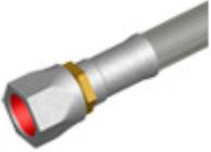
These Teflon\* lined, high pressure hose assemblies are designed specifically for the IMC industry. The hoses are all stainless steel construction and come in several diameters, 3/8" is standard. Rated for use at 6000 psi (4:1 Safety rating), the standard ends are 37 degree female swivels.
